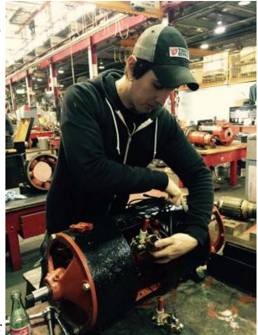
Expert care: Darren Hawe, a 32 year-old second class electrical worker with Local 717 IBEW, repairs a 129MG generator used in the Mattapan fleet of PCC cars at the Everett Shops. Bill Forry photo
