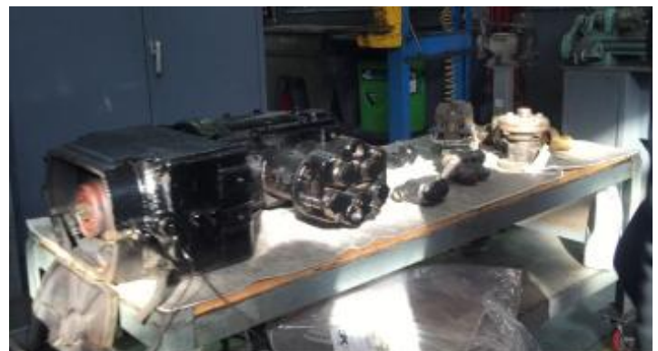
Westinghouse DH10 Air Compressor: An essential component to the PCC cars, the MBTA team has been able to repair this original compressor, but has not had to rebuild them from the ground up— yet. Bill Forry photo
