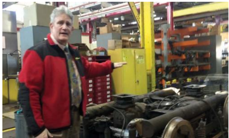
Edward Belanger, maintenance supervisor of the MBTA's subway main repair facility in Everett, explains the components of the “truck” that is the propulsion unit that sits under the Mattapan PCC cars. On average, the MBTA repair crews receive one truck per month to re-build or repair. Bill Forry photo
